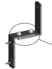
Dual Bracket components are pre-assembled by manufacturer. Do not adjust or remove unless authorized by the manufacturer.
