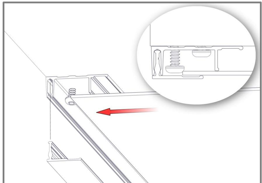
Step 9 - Once planks are installed, finish off the perimeter trims with caps from two-piece sets.
