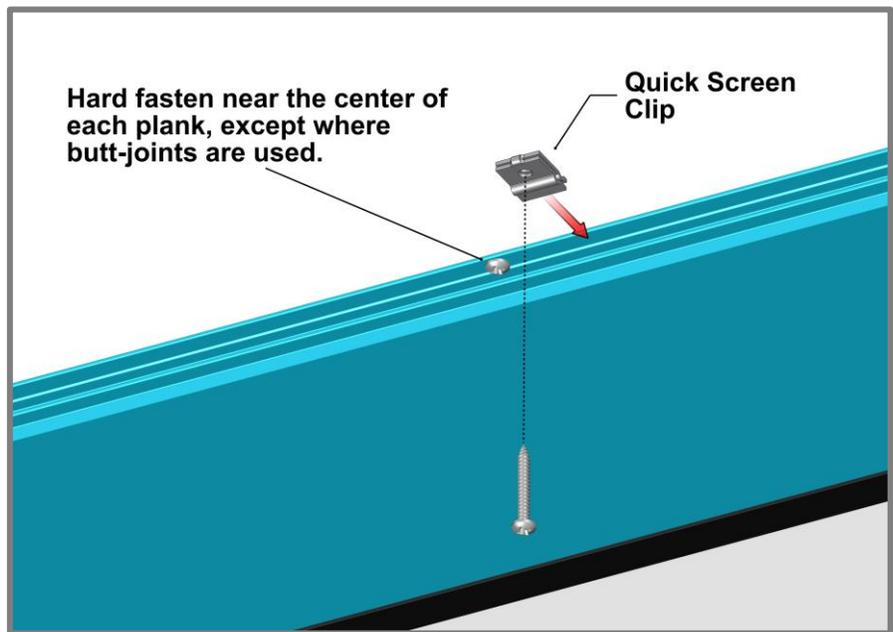
Where anchoring the planks securely can only be achieved over component flanges; split the Quick Screen Clip and use one piece on the front. This will maintain each Planks ability to expand and contract.
