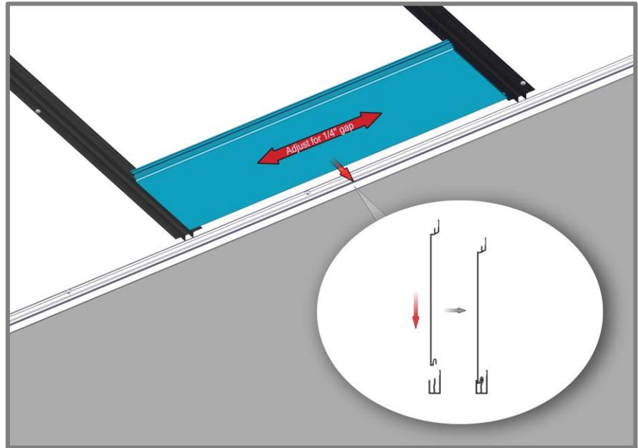
Install Quick Screen Clips every 32" (813mm) O.C. max spacing. Hard fasten only one point near the center of each plank or fasten at the butt-joints where butt-joints are used. Shim Quick-Screen Clips where needed to correct any substrate inconsistencies.
